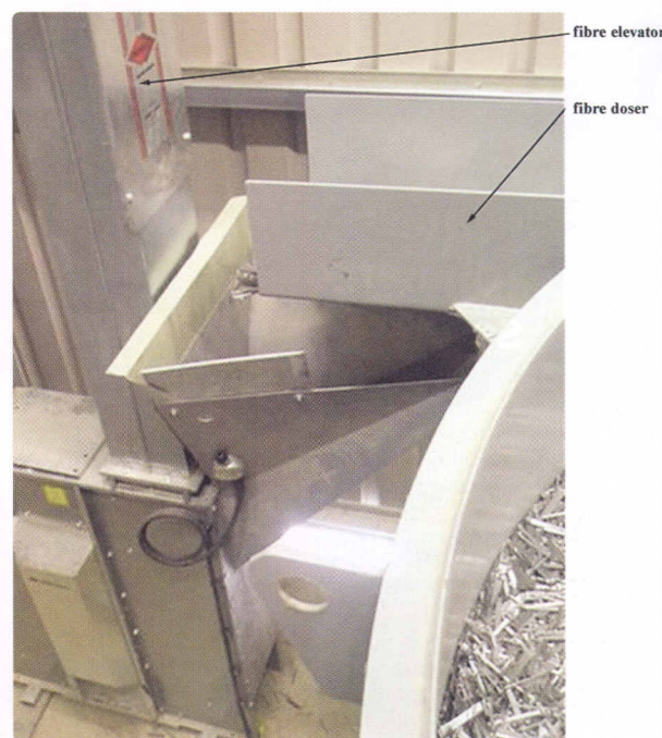
Figure 4 above left: Batching plant at Tarmac after installation of fibre-dosing system.
